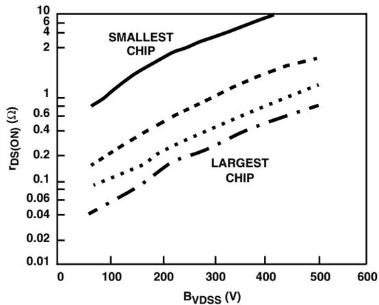
**FIGURE 3. AS CHIP SIZE INCREASES,  $r_{DS(ON)}$  DECREASES**
