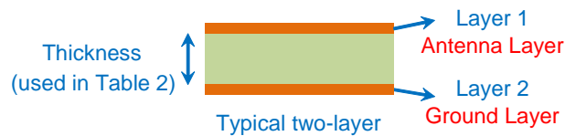
Figure 11. Clarification of PCB Thickness
