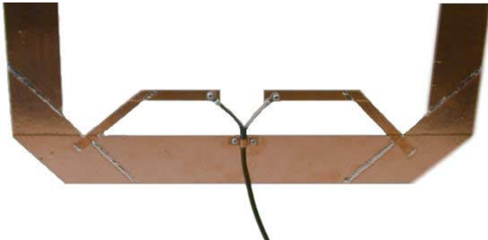
Figure 18. T-Matched Tape Antenna
