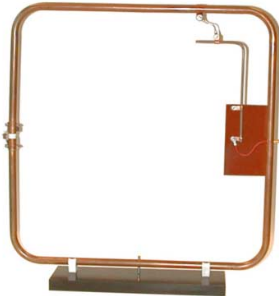
Figure 14. Gamma Matched Antenna
