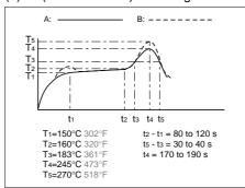
Temperature rise of relay itself may vary according to the mounting level or the heating method of reflow equipment. Therefore, please set the temperature of soldering portion of relay terminal and the top surface of the relay case not to exceed the above mentioned soldering condition. It is recommended to check the temperature rise of each portion under actual mounting condition before use.
