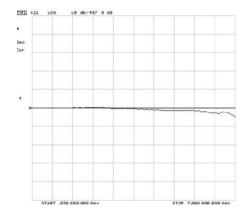
Insertion loss tested to 7 GHz for the CRFReed Relay but with the internal Reed Switch replaced with a bare copper wire. Horizontal full scale: 7.0 GHz. Vertical scale: 10 dB/div referenced from the 0 mark.
