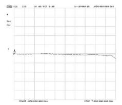
Insertion loss tested to 7 GHz for the CRF Reed Relay. Horizontal full scale: 7.0 GHz. Vertical scale: 10 dB/div referenced from the 0 mark.
